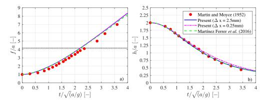
Figure 2: Normalised horizontal position of the dam break front (a) and height at the left wall (b) as a function of normalised time. The dotted black line indicates the shared boundary between regions.
