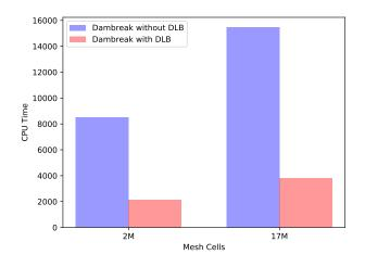
Figure 6: Performance Comparision between Dynamic load balancing and without dynamic load balancing for Dam Break with Obstacle test case
