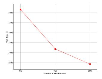
Figure 8: Scaling of the 'dam break with obstacle' test case using wsiFoam solver with 17M mesh cells
