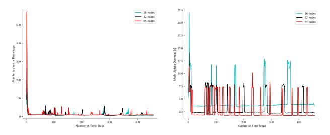
Figure 7: The maximum imbalance (a) and mesh update cost (b) as a function of time step number. These results were obtained for the 17M cell 'dam break with obstale' test case using dynamic load balancing.
