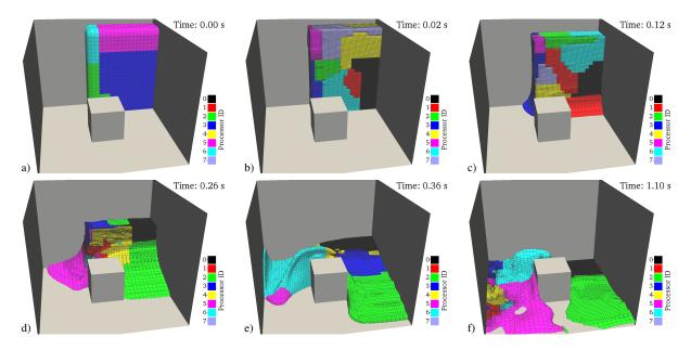
Figure 5: Snapshots of the volume of fluid isosurface ( $\alpha_1 = 0.5$ ) from the dam break with obstacle case using eight processors, adaptive mesh and dynamic load balancing. The colours represent the sections being solved by each processor, and the grey lines show the mesh discretisation.
