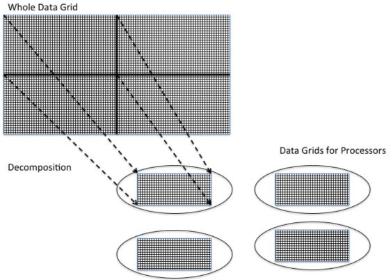
Figure 2 - Breaking up the problem through domain decomposition
